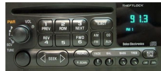
Main AM/FM radio in upper dash (not a separate or slave player)
